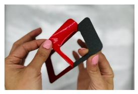
Hold the pieces by the edges to avoid touching the adhesive surface. Peel the RED Protective tape off, place piece in position, align it correctly, and thoroughly press down on the entire surface of each piece to ensure complete adhesion. Repeat this step for all pieces you have.
